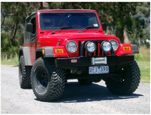
The Multi-fit Winch Bar is specially designed with shorter wings so that it will fit both the Jeep Wrangler YJ and TJ Models, and is also ideal for customers that are fitting larger tyres or would like to maximise their approach angle.
